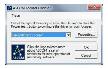
You can then click on the Properties button to access the Setup screen to select the COM port you will be using. If you are using a suitable USB to Serial converter then you need to establish what COM port has been assigned to it first.
