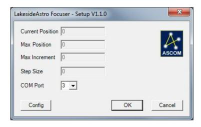
Note that sometimes after the first time that the COM port is changed it does not properly connect to the program. If this is the case ensure that the correct COM port is displayed and shut down the program. After restarting the problem should be resolved and should not re-occur unless the COM port is changed.
