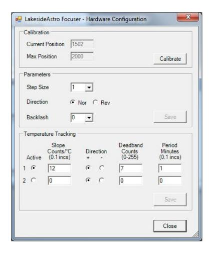
To calibrate the focuser click on the 'Calibrate' button. You will then be asked if you are sure you want to calibrate. If you click on 'Yes' you will see 'REMOTE' displayed on the control unit LCD display and 'IN' and 'OUT' will appear above the two outer buttons.
