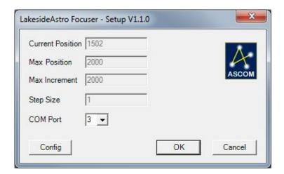
The configuration screen is accessed from the setup screen by clicking on the 'Config' button. This screen can only be accessed when the focuser is connected to a program such as MaxIm, FocusMax or the LakesideAstro Utility program.
